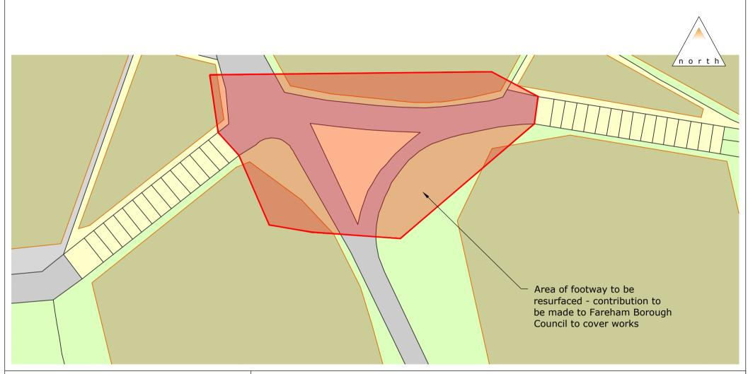
Note: Resurfacing to be of a Hoggin material, comprising of a mixture of clay, gravel and sand. This would allow the surface to be permeable to allow water to drain through. Hoggin surface to be placed on a sub-base.
